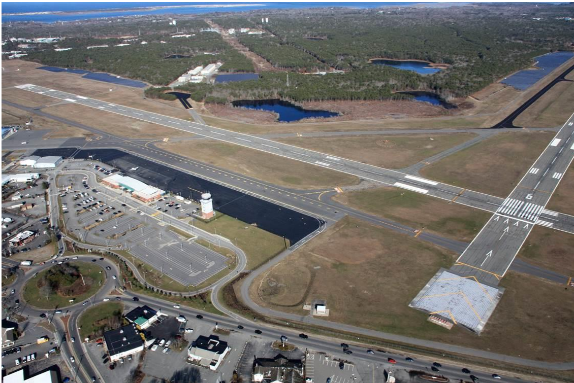
February 2017 Airport Aerial Showing New Terminal Ramp, New Portion of Taxiway Charlie and Both Solar Arrays
