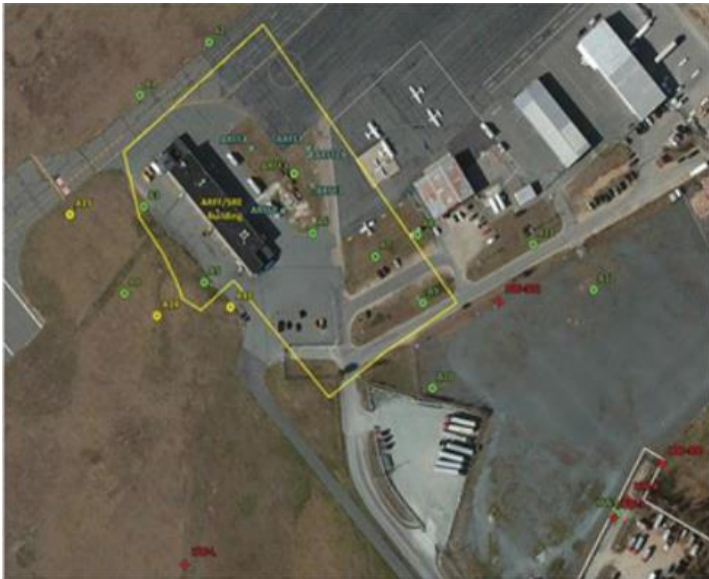
AFFF Truck Storage & Maintenance Site Location noting higher concentrations of PFAS. Turf location north of building chosen by MassDEP for mitigation.
