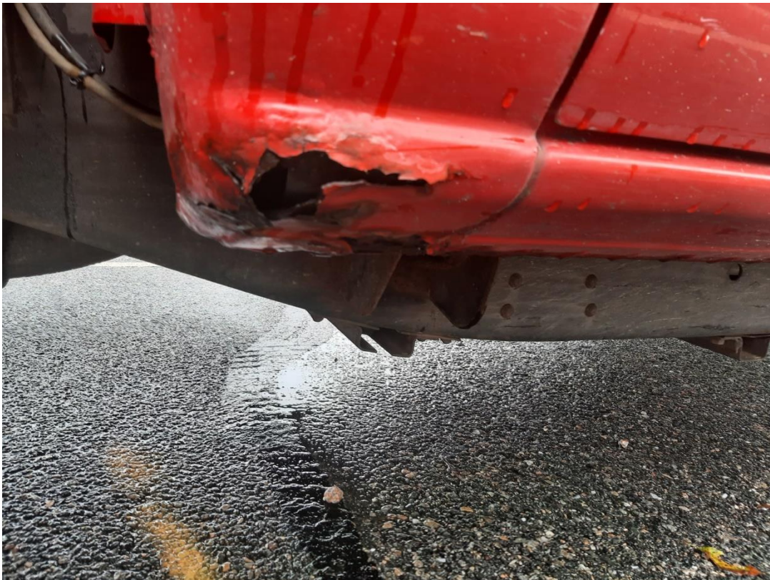
Example of corrosion on Truck 254
